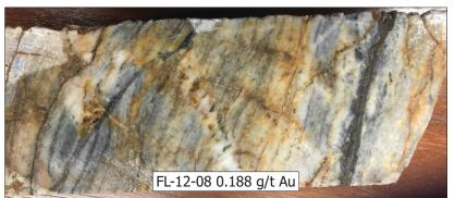
The 2012 drilling intersected numerous narrow (0.7 to 2 m) gold bear ing structures (>1 g/t Au) and broader zones (5-15 m) of elevated arsenic very similar to gold mineralization elsewhere in the White Gold District. All of the drill holes are widely spaced and isolated and there has been no follow-up of the known Au mineralized structures to delin eate their orientation and continuity.
